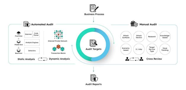
Automated audit ensures high quality of security assessment by finding various attacks quickly and precisely through cooperative analysis between static and dynamic analysis. Our static analyzer analyzes target codes through parsing grammar and verifies constraints through path finding and variable tracking. In dynamic analysis, emulation of target codes is executed in SOOHO's own test network along with fuzzing and concolic execution.
